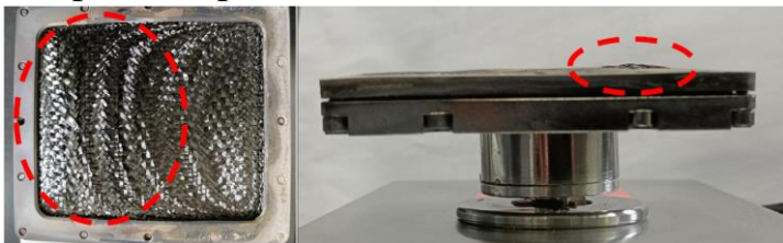
swelling observed on CFRP plate at 10°
