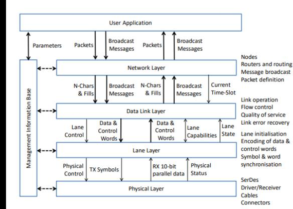
Figure 5-1: SpaceFibre protocol stack - single-lane
