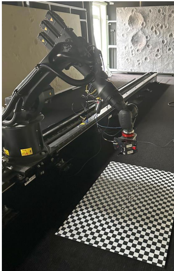
Data acquisition for hand-eye calibration
