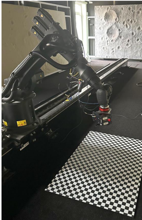
Data acquisition for hand-eye calibration
