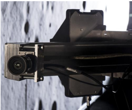
Camera installed on robotic arm
