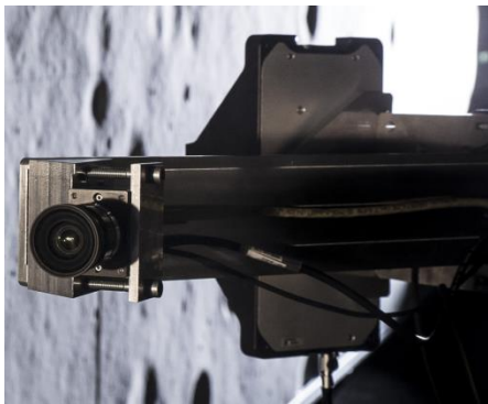
Camera installed on robotic arm
