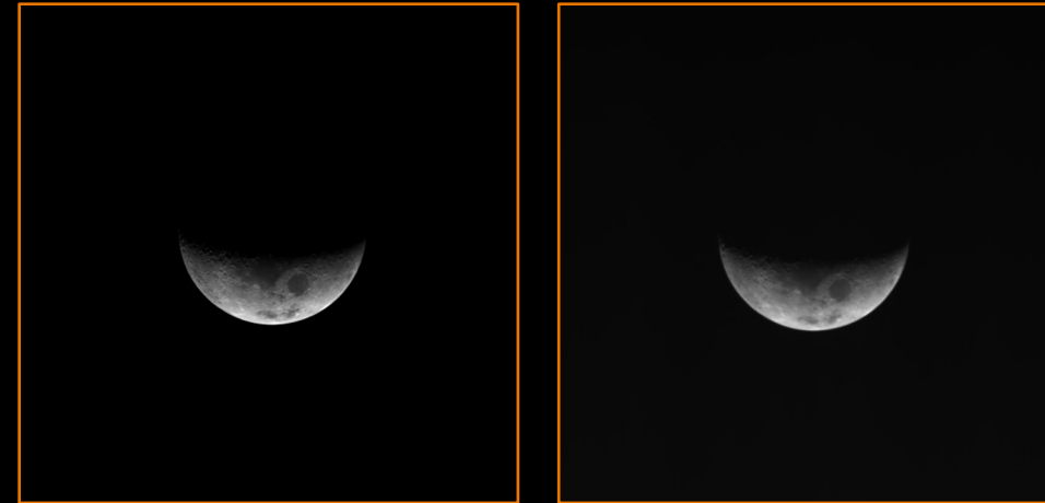
CORTO rendering (left) vs real image (right) at 30 ms exposure time
