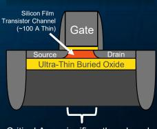
Lattice FPGA in 28nm FD-SOI
