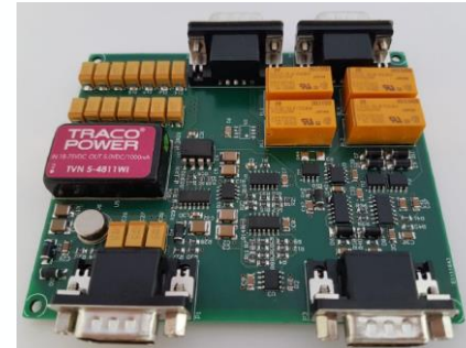
Proof of concept of short-circuit triggering system (left) and short-circuited magnetorquer (right)
