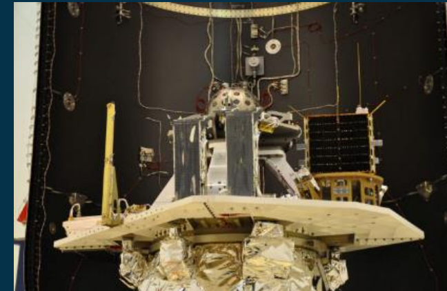
AVUM with LARES-A&H/SS platform. ALMASat and the Cubesats dispensers are also visible.
