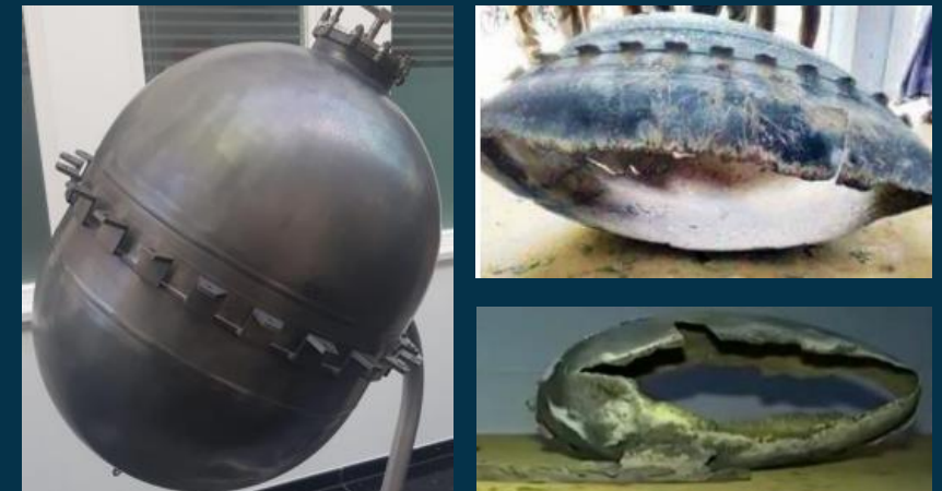
Titanium tank: before (left) and after re-entry (right).
