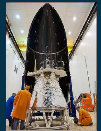
AVUM with LARES-A&H/SS platform. ALMASat and the Cubesats dispensers are also visible.
