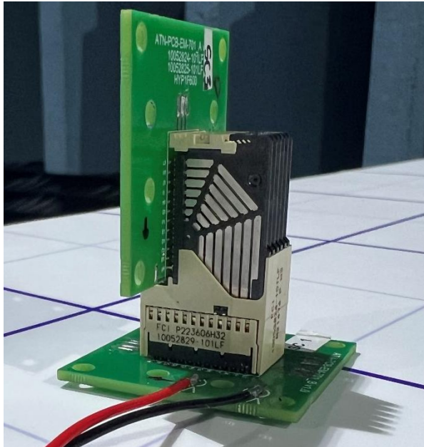
C-D mated connectors before assembly on the vibration test jig
