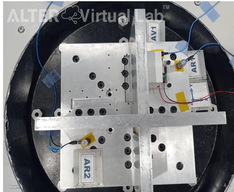
Top view of the connectors assembled on the vibration test jig
