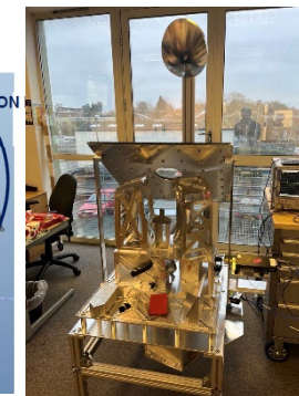
Quasi-Optical Network Breadboard (courtesy Thomas Keating Ltd - UK )
