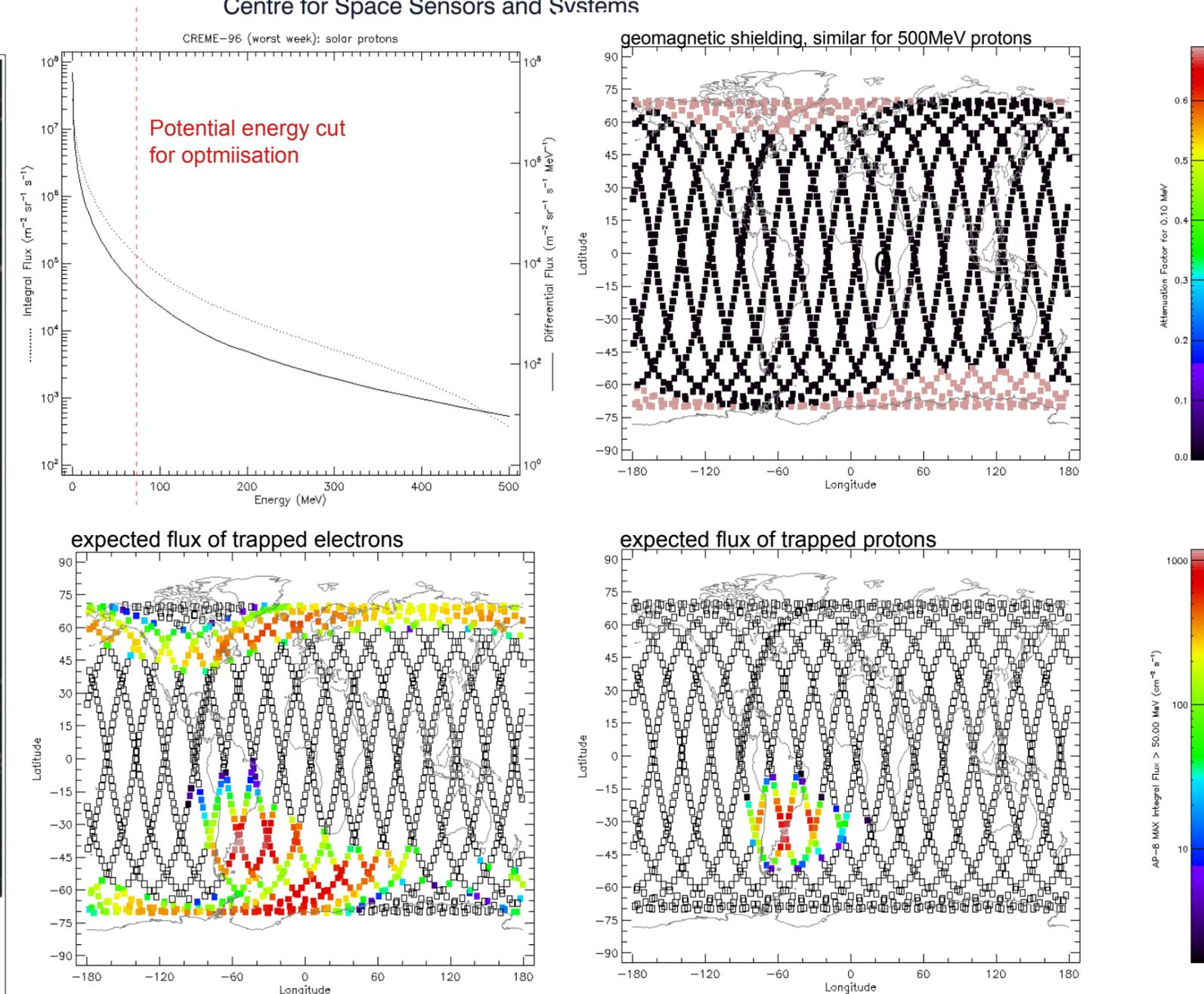
Good understanding of the radiation environment in LEO is essential for the detector design parameters. Tools such as the Space Environment Information System (SPENVIS) are useful for estimating particle fluxes, though various models and tools to ensure accuracy will be reviewed during the mission design phase.
