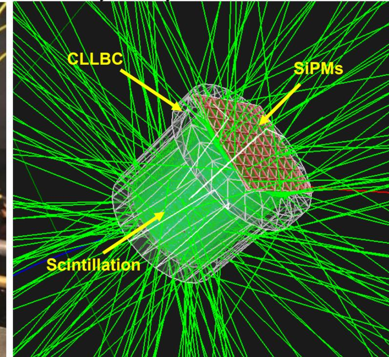
Geant4 simulation of the detector geometry. Scintillation photons are confined within the detector volume.
