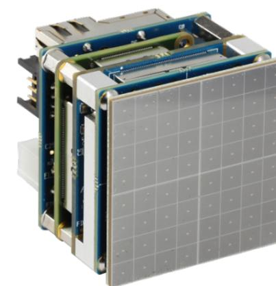
An array of Hamamatsu SiP mounted on top the readout electronics (ROSSPADs)
