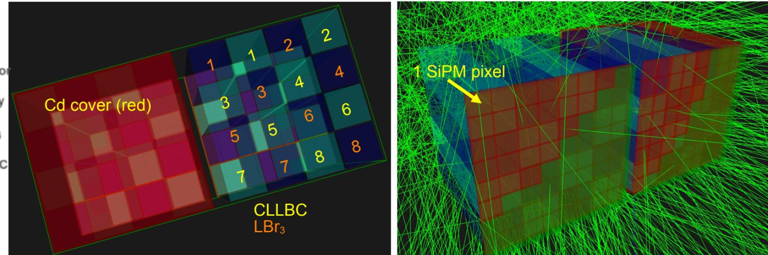
Geant4 based simulation of two detector units, one of which is covered in Cd sheet to filter away thermal neutrons.
