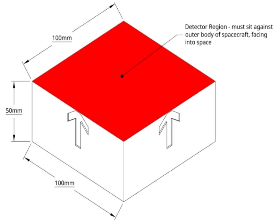
1U payload, consists of two detector units, one zenith and one nadir facing, taking 10x10x10cm space.
