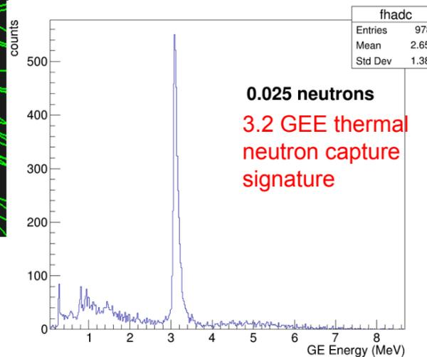
Geant4 results, Top: Energy spectrum for 0.662MeV Cs-137 source, Bottom: Energy spectrum from thermal neutron capture.
