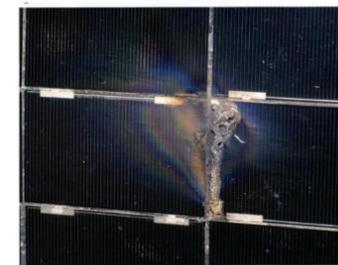
(b) Failure caused by ground ESD arcing
