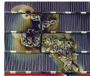
(a) Failure caused by in-flight ESD arcing
