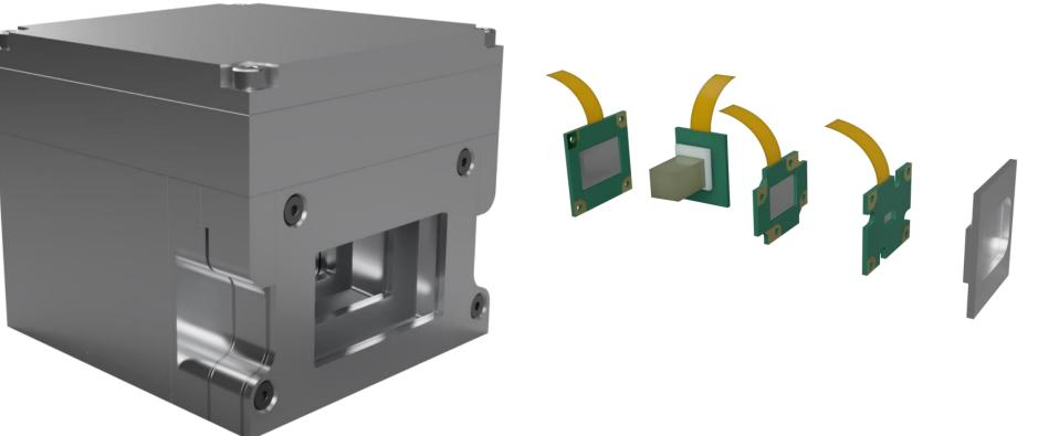
REPE measures electrons and protons using a stack of three silicon detectors and a scintillator with photodiode readout.
