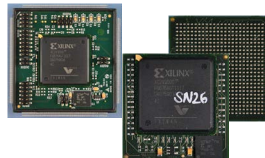
Prototype Adapter Boards with same footprint as RTAX FPGAs
