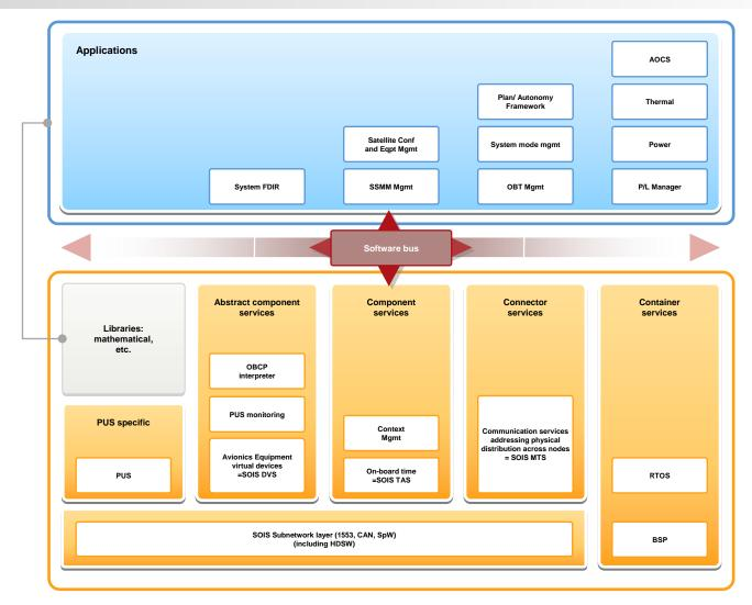
Application level hosts the components of the functional chains
