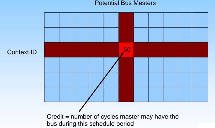
On a multi-core system the arbiter schedule may need to be linked to/controlled by a single "master" or "root" core.
