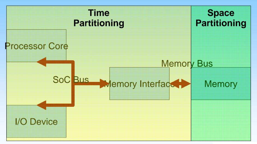
Processor core, SoC bus, all interfaces treated as a single resource
