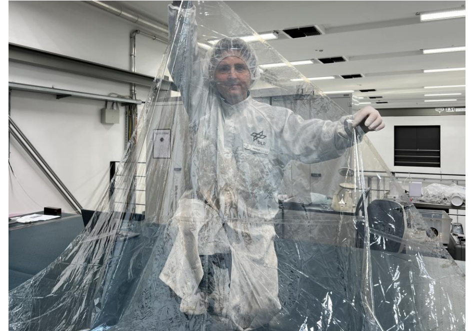
First transparent sail segment breadboard (ITO-coated FEP)
