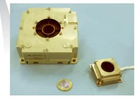
Modern **Sun sensors** are already twocomponents' units, with APS and ASIC. The huge amount of signal, the non stringent accuracy requirements and the pinhole concept make the **miniaturization within reach.**
