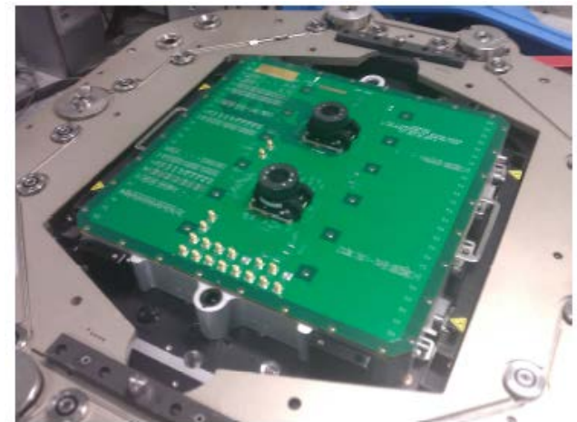
Quator automated test equipment board (ATE) ST Integraflex tester
