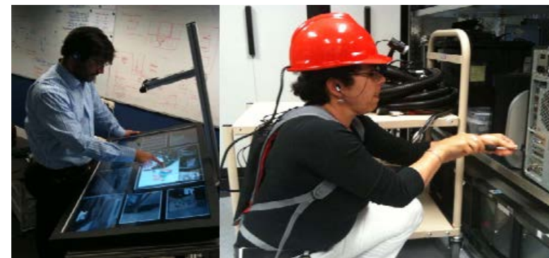
ReMoTe, remote guiding system - hand gesture communication in mining industry (Alem et al., 2011).
