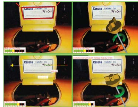
(De Crescenzo et al., 2011) AR system for airplane maintenance.
