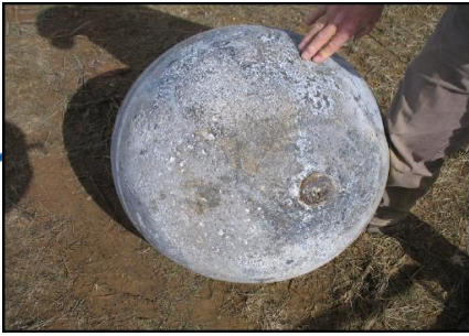
Pressurant tank found in Colorado in March 2011 and tentatively linked to a Zenit launch vehicle stage.
