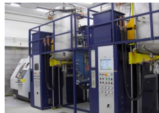
Advanced high temperature furnaces for pyrolysis and siliconization
