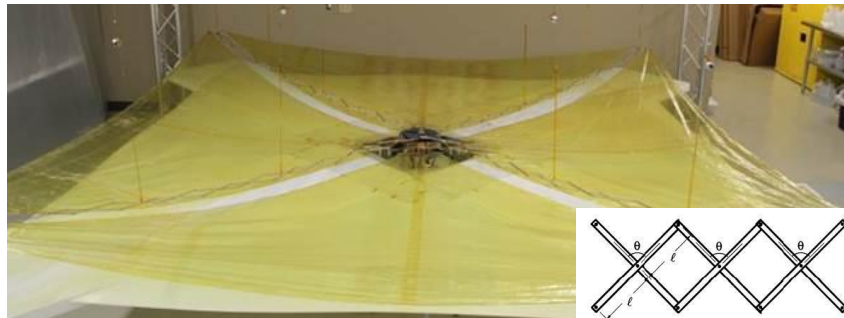
dragNET de-orbit system using pantograph type deployable booms for support of the sails (Courtesy of MMA Design)
