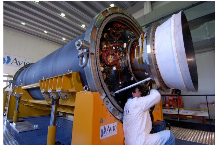
DeltThe thrust vector control system of the Zefiro 23 engine, part of the Vega launcher Courtesy of ESA
