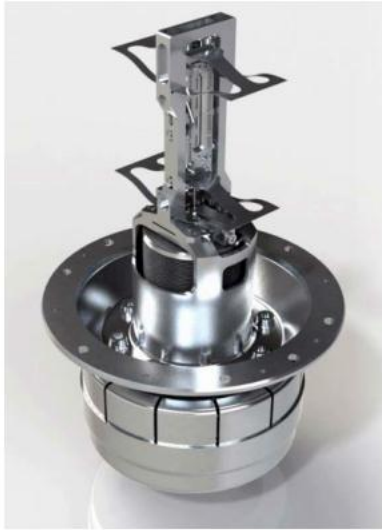
Slit-Change Mechanism (SCM) part of the SPICE instrument on board of Solar Orbiter
