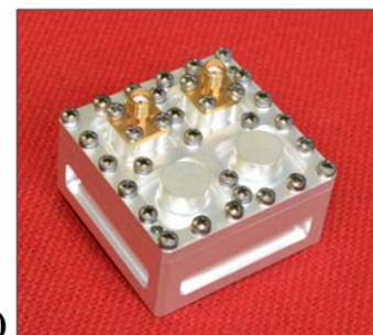
Figure Manufactured filter prototype: open case with silver-plated dielectric rods (a), final version of the filter (b)
