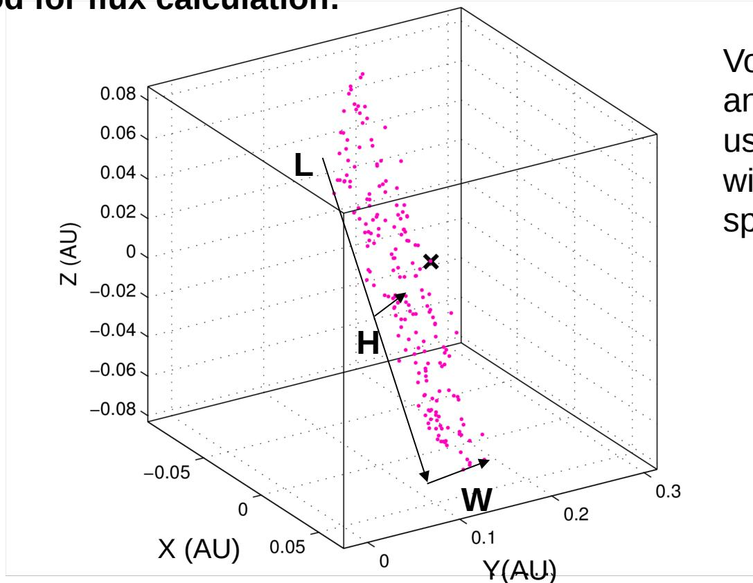
Volume calculated as an elliptical cylinder using trail dimensions within 0.1AU of the spacecraft
