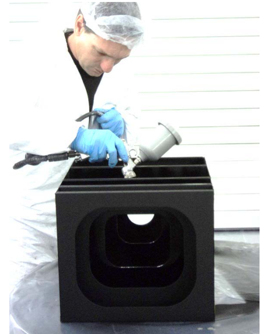
Optical baffle - stellar diurnal sensor of the PILOT experiment ( stratospheric balloon) MAP® AQ PU 1
