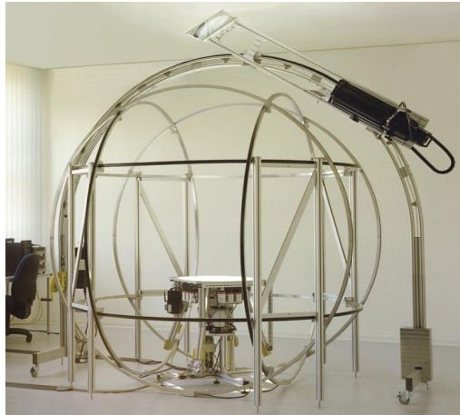
Fig. 6. AFWs attitude control test facility
