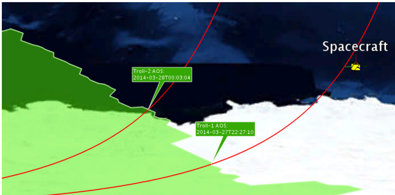
Fig. 5. Spacecraft reaching the point of AOS at the Troll ground station. Note ground track over two orbits represented as a red line. Troll ground station visibility mask is represented as a green polygon. Point of AOS is indicated by a green text box which indicates the number of the pass as well as the time of AOS.
