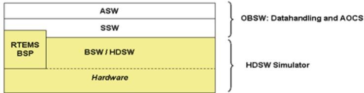
Figure 7: OBC Simulator Component (1/2): implementation based on HDSW Simulator and ASW.
